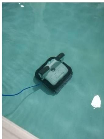
When pulling cleaner out of water suspend the cleaner above water for about 10-15 seconds to empty the water inside. Please holds the top handle only, never pull the cable.
